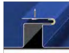
Typical 1 Reveal For 12" Panels
