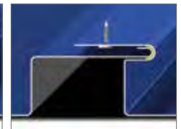
Custom Reveal For 12" Panels up to 3"
