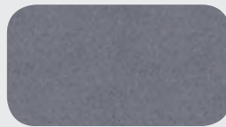
WEATHERED GALVALUME SR:0.30 E:0.79 SRI:27
