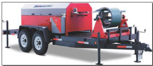
Figure 2-9 Mobile Roll Former Used “On-Site.”
