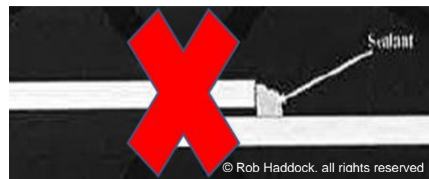
Figure 15-15 Butyl Sealant Should NOT be Externally Applied
