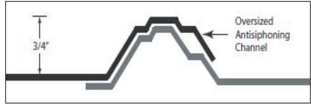
Figure 5-7 Typical Trapezoidal Rib with Overlap Seam
