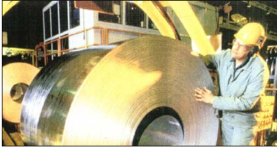
Figure 5-3 Large Coils of Sheet Metal Allow Larger Roof Panels to be Produced
